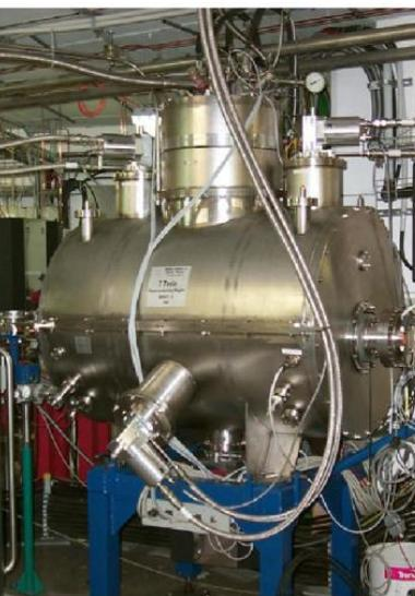
Fig. 2-4 Photo of 7 Tesla WLS inserted into BESSY-2 straight section.
